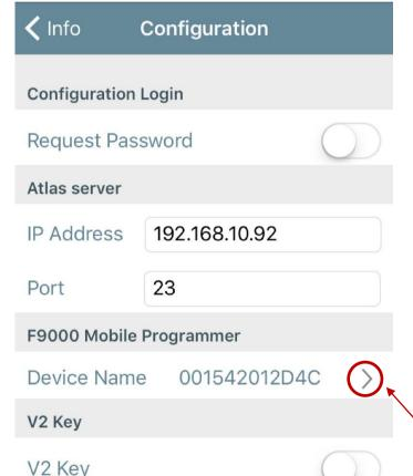
Set the IP Address and Port defined on the Ethernet Gateway (see its configuration) if you use the device in your network.
