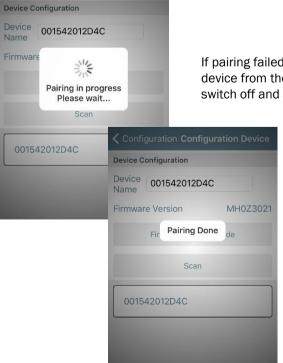
If pairing failed, before training again, remove the device from the bluetooth list (if exist) and then switch off and switch on the bluetooth.
